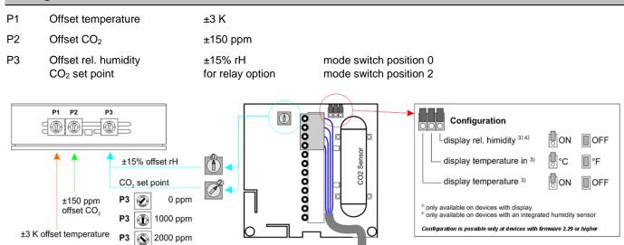
For configuration set mode switch to the appropriate position and then choose offset or set point using P1 to P3. With changing P1 to P3 the value is stored in the device.
